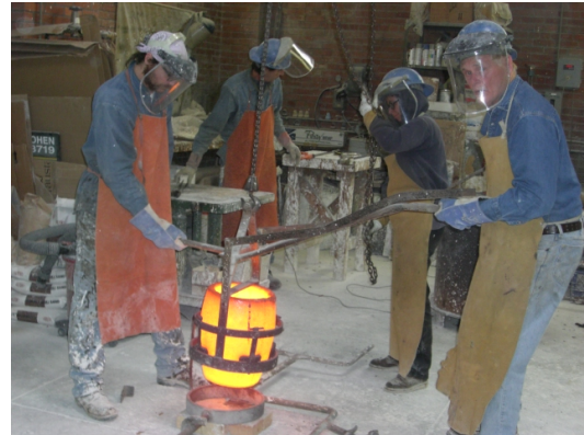
3. Bronze is melted for casting
